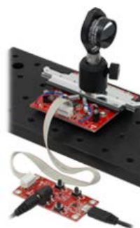
Click for Details [APPLIST] [APPLIST] An ELL10K Linear Stage Bundle used to position a hollow roof mirror in an optical delay line.
