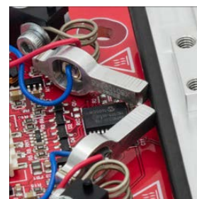
Click to Enlarge Red and blue wires deliver power to the motors, whose aluminum tips contact the black plastic strip at the edge of the linear stage.
