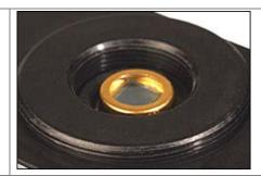
A close up picture of the front of a DET series biased photodiode detector with the SM1T1 removed. The external SM1 and internal SM05 threading on the detector housing can be seen in this image.
