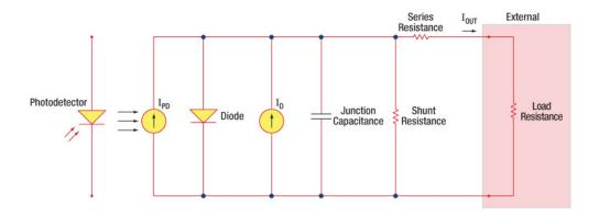
Figure 1: Photodiode Model
