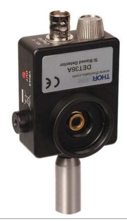
DET series detector mounted horizontally on a TR series post. Notice how the on/off switch is easily accessible from the top and the electrical connection comes in perpendicular to the beam path.
