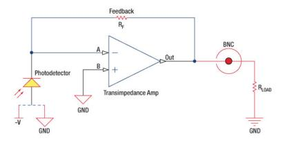
Figure 3: Amplified Detector Circuit
