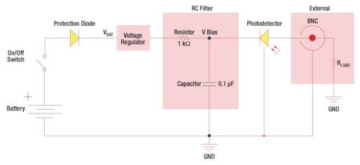
Figure 2: Reverse-Biased Circuit (DET Series Detectors)
