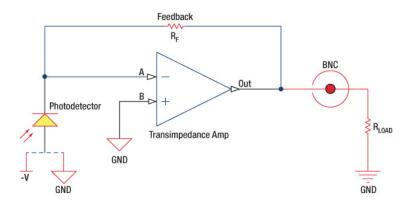
Figure 3: Amplified Detector Circuit
