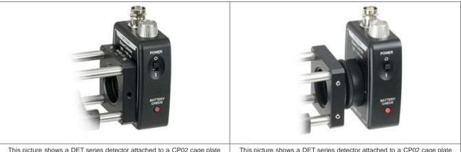
This picture shows a DET series detector attached to a CP02 cage plate after removing the SM1T1. The retaining ring from the SM1T1 was used to make the orientation of the detector square with the cage plate. This picture shows a DET series detector attached to a CP02 cage plate using an SM1T2 adapter in addition to the SM1T1 that comes with the DET series detector.
