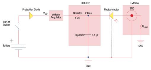
Figure 2: Reverse-Biased Circuit (DET Series Detectors)
