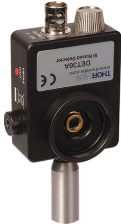
DET series detector mounted vertically on a TR series post. This image shows the VBIAS OUT button that can be pressed and held to check the battery's charge (this process is described in the manual).
