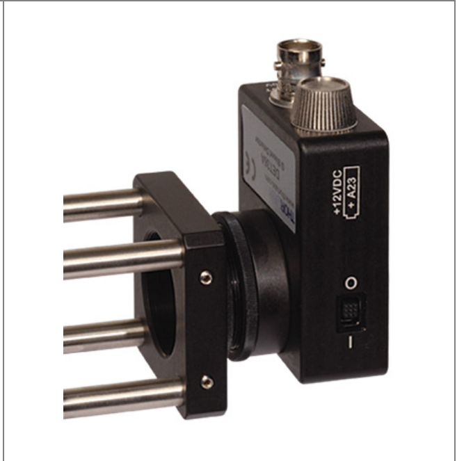
This picture shows a DET series detector attached to a CP02 cage plate using an SM1T2 adapter in addition to the SM1T1 that comes with the DET series detector.
