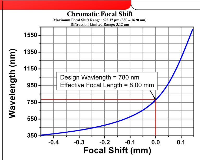
Table showing the focal length at various laser line wavelengths
