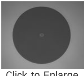
Click to Enlarge Undamaged Fiber End
