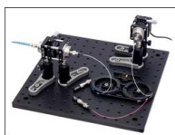
Click to Enlarge Setup to Measure Extinction Ratio of a 1550 nm PM Coupler
