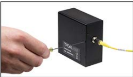
Click to Enlarge Use a 0.05 hex to tighten the setscrew that holds the included fiber collimator in place (fiber patch cable not included).
