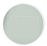
The photograph above is a protected aluminumcoated mirror after LIDT testing. In this particular test, it handled 0.43 J/cm² (1064 nm, 10 ns pulse, 10 Hz, Ø1.000 mm) before damage.
