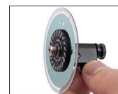
Figure 4: Insert the Front Assembly into the Mount and Screw on the Rear Thumbscrew
