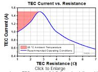
The maximum TEC current of 1.5 Å can be delivered into a load resistance of 2.66  $\Omega$  under the recommended operating conditions. At a higher load resistance, the maximum output current drops due to the limit of the compliance voltage. The maximum output current at lower than 2.66  $\Omega$  load resistance (shaded range) depends on environmental conditions.
