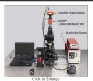
A hyperspectral imaging system built using Thorlabs' Cerna<sup>™</sup> Microscopy Platform, KURIOS-VB1 Tunable Bandpass Filter, and 1501M-GE Monochrome Scientific Camera. Several components shown here were modified from their stock configuration.
