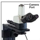
Click to Enlarge This Cerna™ microscope includes trinoculars with a 1X camera port for widefield viewing.
