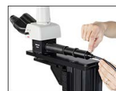
Click to Enlarge The back of the epi-illuminator includes a removable, SM1-threaded adapter that accepts liquid light guides.
