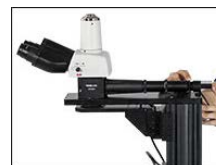
Click to Enlarge A Thorlabs' Mounted LED can be threaded into the epi-illuminator and secured using the included locking ring.
