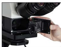
Click to Enlarge The front cover of the epi-illuminator is removed by unscrewing two M2 screws to install a filter cube (not included). Magnets on the cover and the housing ensure that the filter cube is positioned correctly when the door is replaced.
