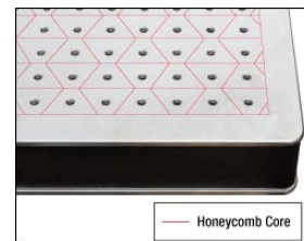
Click to Enlarge Outline of the honeycomb core location on an optical breadboard. The core does not intersect with any screw holes, allowing for a maximum screw depth of 54 mm.
