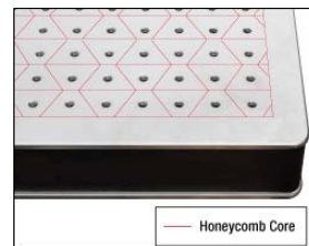
Click to Enlarge Outline of the honeycomb core location on an optical breadboard. The core does not intersect with any screw holes, allowing for a maximum screw depth of 54 mm.
