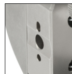
Click to Enlarge The POLARIS-K1T8 has Two Ø2 mm Dowel Pin Holes by Each #8 (M4) Counterbore for Alignment
