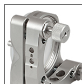
Click to Enlarge POLARIS-K2F with POLARIS-LN1 lock nut installed. Two dowel pin holes and #8 counterbores are visible on the side of the mount.
