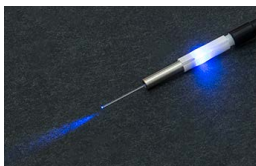
Click to Enlarge Improperly connected cannula and patch cable, showing an air gap and light leakage.
