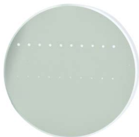
The photograph above is a protected aluminum-coated mirror after LIDT testing. In this particular test, it handled 0.43 J/cm 2 (1064 nm, 10 ns pulse, 10 Hz, \varnothing 1.000\text{ mm} ) before damage.
