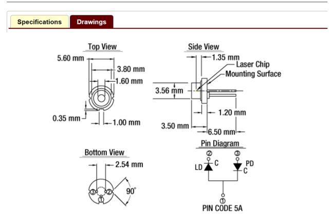
M5-905-0100 - 905 nm, 100 mW, Ø5.6 mm, A Pin Code, Laser Diode
