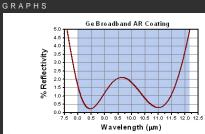
Shown above is a theoretical graph of the percent reflectivity of the AR coating as a function of wavelength. The average reflectivity in the 8 - 12  $\mu m$  range is <1.5%. The blue shading indicates the recommended usage range for these Ge plano-convex lenses.
