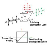
Polarizing Beamsplitters - Thorlabs' polarizing plate and cube beamsplitters split randomly polarized
