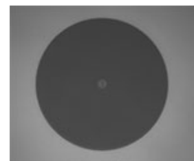
Click to Enlarge Undamaged Fiber End
