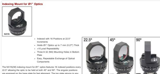
22.5° allowing the optic to be held at both 45° and 90°. The angular positions are engraved on the base plate for fast alignment. The top plate returns to any given position, indicated with an engraved witness line, with a repeatability of better than 10  $\mu$ rad. This mount is ideal for redirecting a laser to multiple targets on an optical table, as well as for precise switching of shared laser systems.
