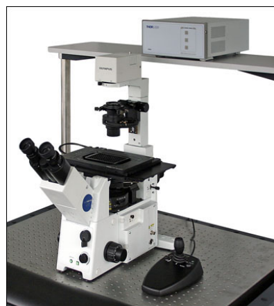
A typical XY stage setup is comprised of an MLS203 stage, BBD202 XY Stage controller, MJC001 2-Axis Joystick, and inverted Olympus microscope.
