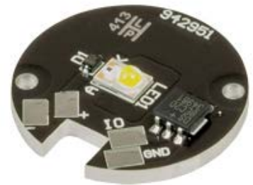
M565D2 565 nm LED, Power Output > 880 mW
