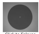
Click to Enlarge Undamaged Fiber End
