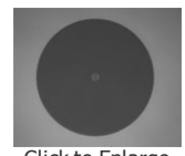
Click to Enlarge Undamaged Fiber End
