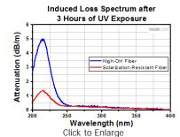
Comparison of Loss Induced by Solarization in 1 m of High-OH fiber compared to Solarization-resistant fiber after 3 hours of UV exposure
