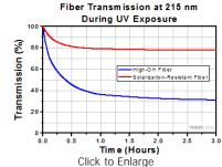
Solarization-Resistant Fiber Transmission Compared to Standard High-OH Silica Fiber (25 W Deuterium Lamp; 1 m Fiber Length)
