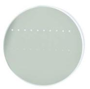
The photograph above is a protected aluminum-coated mirror after LIDT testing. In this particular test, it handled  $0.43 \text{ J/cm}^2$  (1064 nm, 10 ns pulse, 10 Hz,  $\emptyset 1.000 \text{ mm}$ ) before damage.
