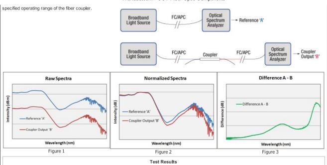
Each possible optical path is analyzed for the wavelength dependence of the coupling ratio, yielding 4 traces for each coupler as shown in the sample plots below. Every OCT fiber coupler placed in inventory is tested to ensure that it meets the criteria listed below.
