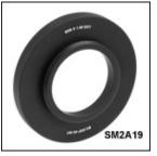
Our SM2A19 adapter is ideal for making any of our BE03M or BE05M beam expanders compatible with the SM2 (2.035"-40) thread standard found on many of our products including our  $\emptyset$ 2" lens tubes and 60 mm cage systems. The adapter features internal SM2 threads and external M36 x 1.5 threads.
