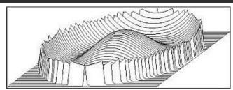
Left: Typical wire grid plot of the wavefront distortion of a Gaussian beam that has propagated through a BE series Gaussian beam expander. See the table below for the calculated peak-to-valley wavefront distortion value and the RMS wavefront distortion value for each BE series beam expander at its design wavelength.
