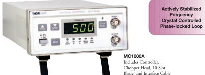
The MC1000A Optical Chopper, which includes a 10-slot (36°) chopper blade (MC1F10), is a precision instrument system utilizing advanced features to meet the most demanding applications. The MC1000A features a microprocessor control and a crystal stabilized phase-locked loop (PLL) motor control for ultimate chopping stability and drift-free performance.
