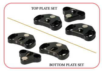
The KBS98 kinematic seats can be used to convert any breadboard into a kinematic platform that can be removed and replaced with a high degree of accuracy. Two of the three seats of each set (top and bottom) have elongated slots to allow the seats to all point to a common center in the middle of the breadboard.
