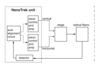
Block Diagram: With one fiber fixed and the other mounted on a piezo-actuated stage capable of moving the fiber perpendicular to its end face, the NanoTrak<sup>TM</sup> controls the position of the moving fiber. The NanoTrak's autoalignment circuit controls the position of the fiber as it optimizes the efficiency of the butt-coupling. In many applications, a planar waveguide or other device replaces one of the fibers; however, the basic principles remain the same.
