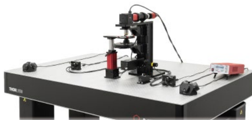
This DIY hyperspectral imaging system is built on Thorlabs' Cerna Microscopy Platform. Key components include the previous-generation KURIOS-VB1 Tunable Bandpass Filter, the CS126MU Monochrome Scientific Camera, and our MNWHL4 Neutral White Mounted LED.
