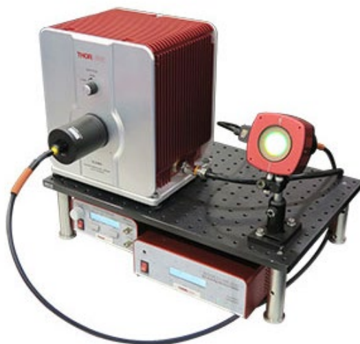
The SLS401 Xenon Arc Light Source coupled using a liquid light guide to our KURIOS-WL1/M Tunable Filter. The Ø35 mm clear aperture within the SM2-threaded housing is visible.
