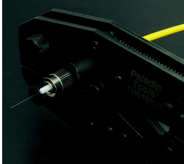
Figure 13 Fixing the crimp sleeve with Thorlabs' Crimp Tool (Item # CT042).
