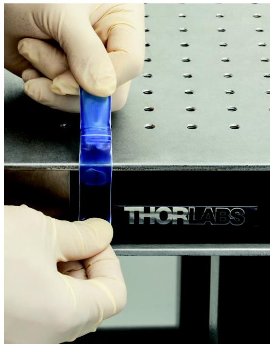
Figure 10 Mixing the epoxy (Item # F112).
