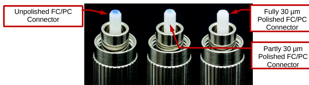
Figure 23 Three FC/PC connectors, from left to right, showing an unpolished, partly polished, and completely polished fiber using the 30 \mu m polishing film.
