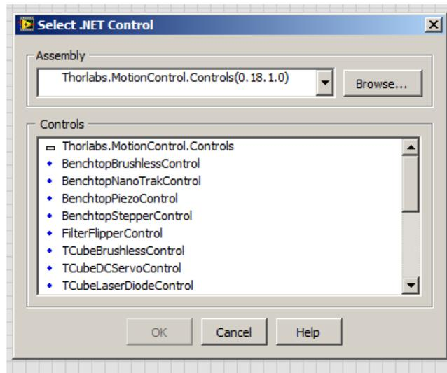
7) From the list displayed, select the control type applicable to the hardware unit you want to load. For example, to insert a T-Cube DC Motor Control object select **TCubeDCServoControl**. Similarly, to insert a Benchtop Brushless DC Motor Control Object, select **BenchtopBrushlessControl**.
