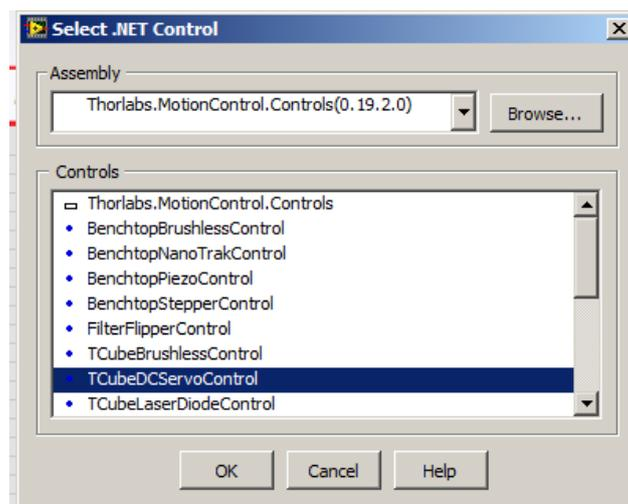
**Note:** In LabView the **TCubeDCServoControl** control represents the .NET control used to interface with DC servo motor controller hardware. Other hardware types have their own .NET controls as shown in the list above.
