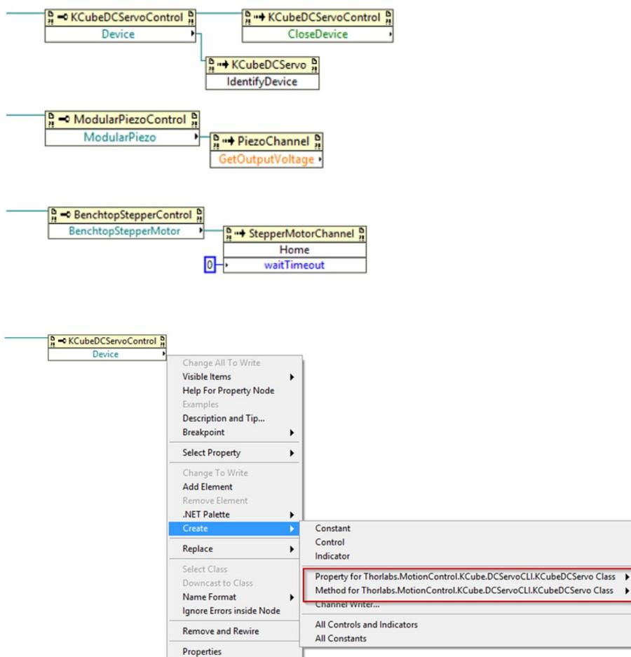
For a 2-channel device such as a BSC202 benchtop stepper motor controller you require two .NET objects on your front panel, one for each channel. To select the channel, add the 'ChannelNumber' element to the BenchtopStepperControl property node & add the channel number.
